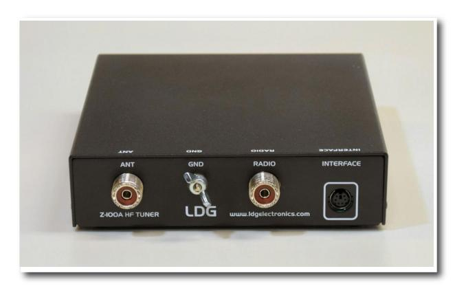
The rear panel of the Z-100A features four connectors.
